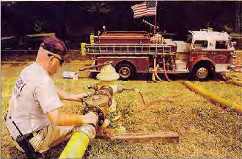
Above, Clint Beem, a Shelby Firefighter, monitors a jury-rigged system that draws water from the City of Kings Mountain through the Cleveland County water system to Shelby. Using the fire truck as a pumping station, 370 gallons per minute are processed.
